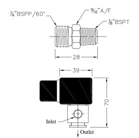
Solenoid Valve 240VAC x <sup>3</sup>/<sub>64</sub>" Orifice 730016
